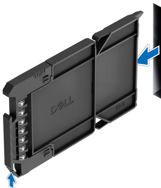
Figure 60. Removing an EDSFF E3.S drive blank
