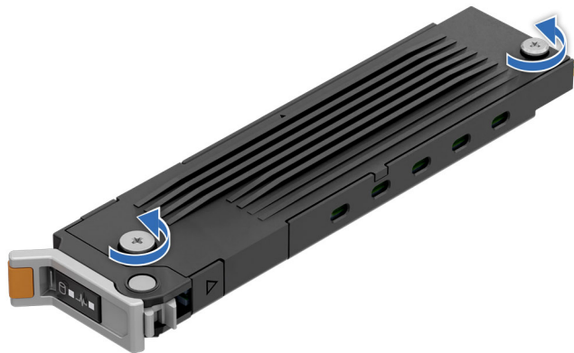
Figure 163. Loosen the top cover captive screws
