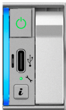
Figure 11. Right Control Panel (RCP) - Primary of R670
