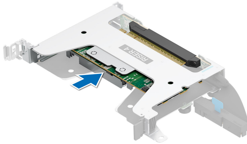
Figure 200. Installing an LP expansion card into the riser 4
