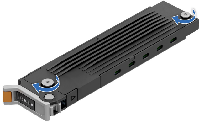
Figure 228. Tighten the top cover captive screws
