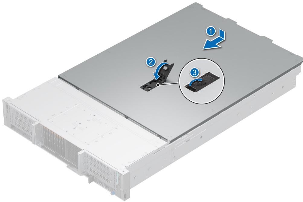
Figure 35. Installing the system cover
