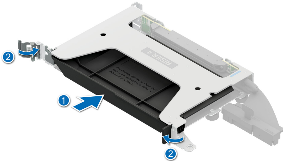
Figure 168. Installing the PCIe blank
