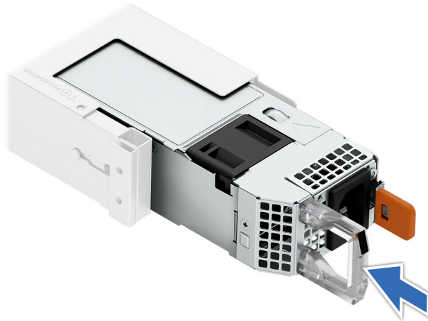
Figure 256. Installing a power supply unit
