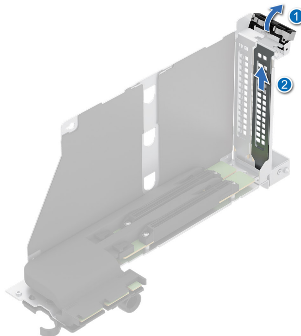
Figure 174. Removing the filler bracket
