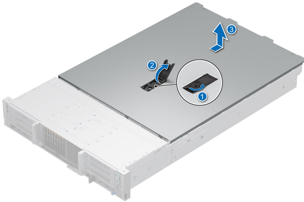
Figure 34. Removing the system cover
