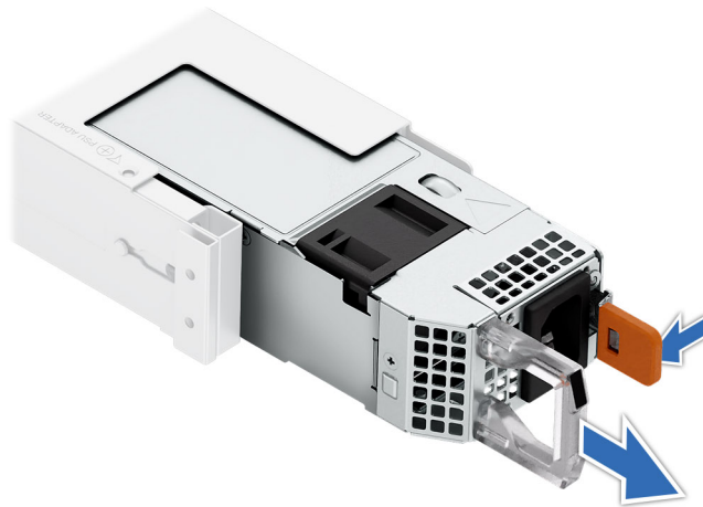
Figure 255. Removing a power supply unit
