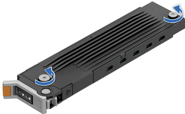
Figure 187. Loosen the top cover captive screws
