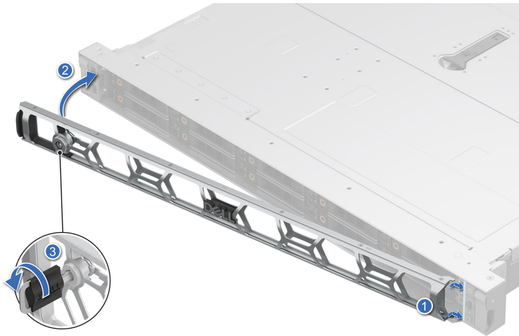
Figure 34. Installing the front bezel
