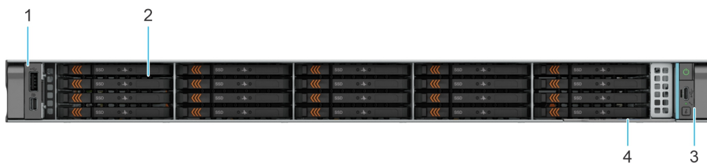
Figure 8. Front view of 20 x EDSFF E3.S Gen5 NVMe + rear 2 x EDSFF E3.S Gen5 NVMe system
