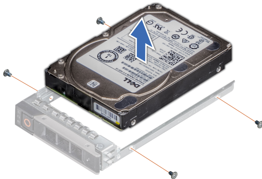
Figure 49. Removing the SSD drive from the drive carrier
