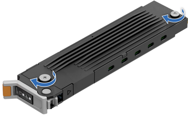
Figure 130. Tighten the top cover captive screws
