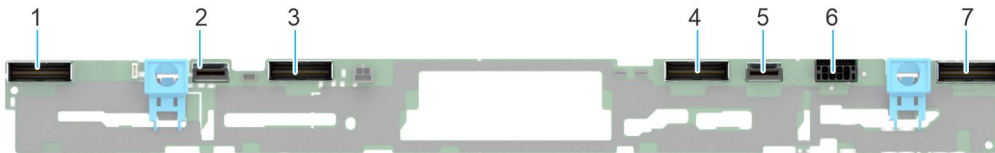
Figure 49. 8 x 2.5-inch Universal drive backplane
