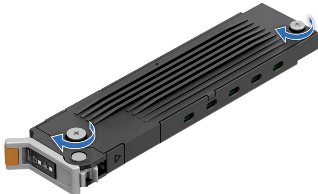
Figure 145. Tighten the top cover captive screws
