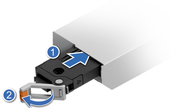
Figure 146. Installing the BOSS-N1 DC-MHS card carrier
