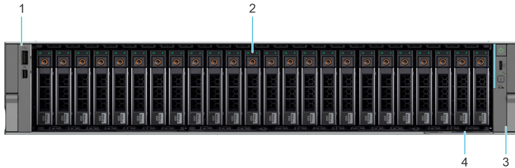
Figure 9. Front view of 24 x 2.5-inch SAS/SATA drives system
