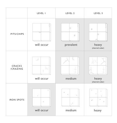
**Unglazed tiles:** Zio & Sons unglazed zellige tiles are rated 'level 2 prevalent' for pits/chips, and 'level 1 will occur' for cracks'.
