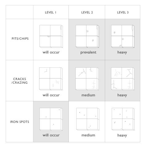
**Unglazed tiles:** Unglazed (Natural) zellige tiles are rated 'level 2 prevalent' for pits/chips, and 'level 1 will occur' for cracks.
