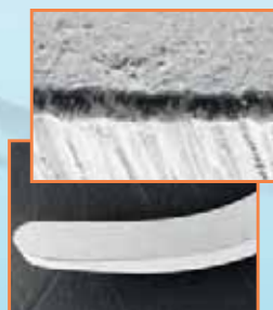
Cutting edge of the LM Sharp Diamond™ curette and the magnification of the edge after the test.
