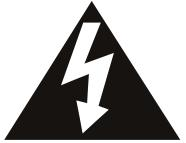
THIS SYMBOL IS INTENDED TO ALERT THE USER TO THE PRESENCE OF NON-INSULATED "DANGEROUS VOLTAGE" WITHIN THE PRODUCT'S ENCLOSURE THAT MAY BE OF SUFFICIENT MAGNITUDE TO CONSTITUTE A RISK OF ELECTRIC SHOCK TO PERSONS.
