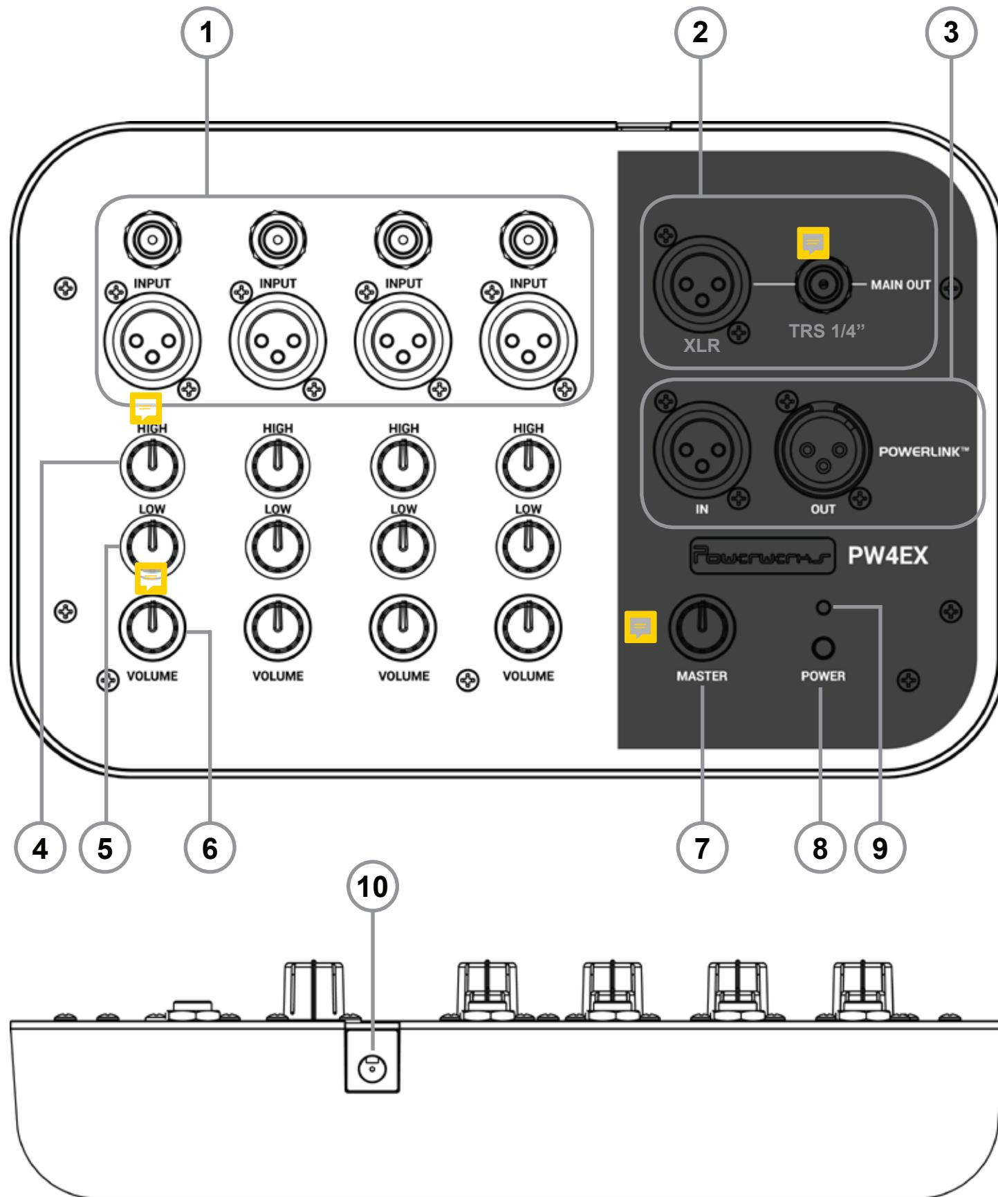
**1. INPUT:** This is where you may plug in microphones, instruments, keyboards, drum machines and other audio devices.
