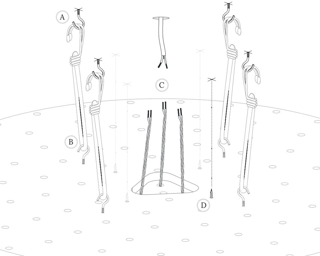
Above is a diagram detailing how the Flock Chandelier is secured to the ceiling and connected to the power supply using the bungees provided to aid installation. The bungees take the weight of the chandelier whilst the electrical connection is being made.
