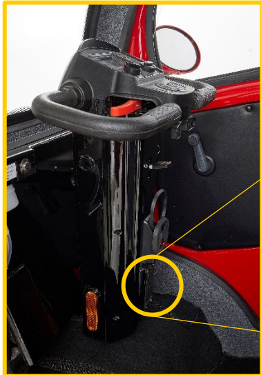
Figure 25 - Fuse box location
