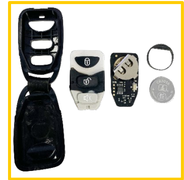
Figure 10 – Central Locking Fob (Batteries)
