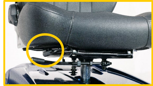
Figure 6 – Pull black handle to adjust the backrest
