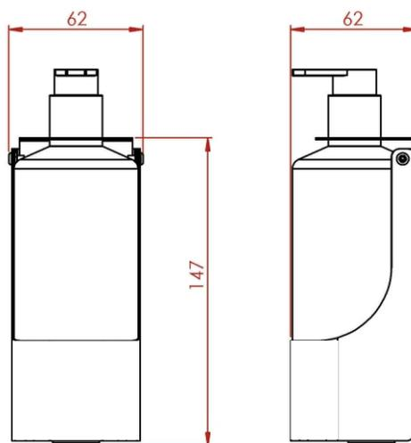
Height: 147mm Width: 62mm Depth: 62mm Weight: 0.5Kg Capacity: x1 250/300ml Bottle
