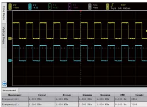
Measure 1 KHz, 2.5 Vpp square waveforms by the measurement function.
