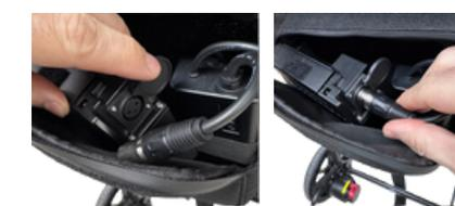
Connect the power cable to the battery by sliding the port cover & inserting power cable.
