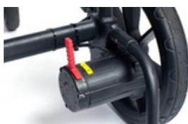
The red brake levers are set in the forward position which engages the motor. For free-wheel mode, pull both levers into the backward position.
