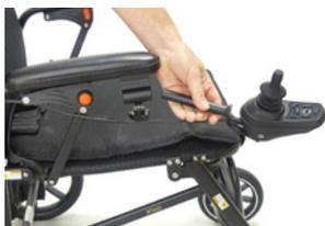
Insert the joystick rod under the armrest and tighten the knob very securely.
