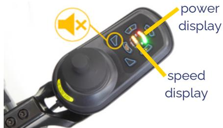
The handset controller features buttons for adjusting speed, with 5 power levels and 5 speed settings (1 = low, 5 = high).
