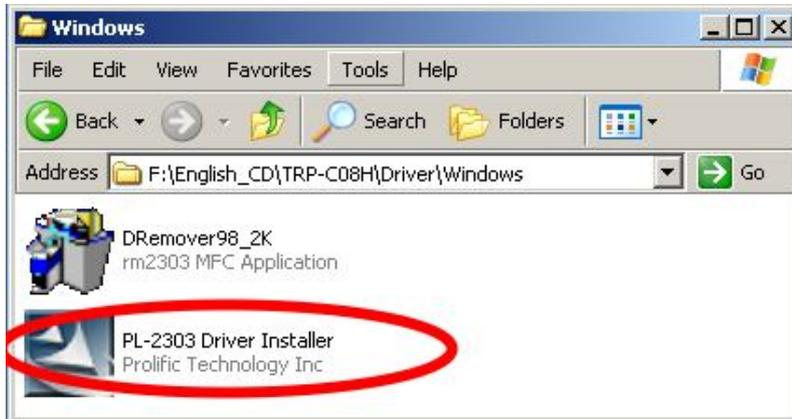
**Step1.** Double click PL2303 Driver Installer” the installShield Wizard screen will appear. The Wizard will guide you to complete the installation.
