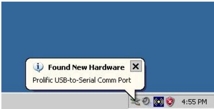
5. After installation user may verify if TRP-C08 was properly installed by Click Start – Setting -- Control panel -- double click system icon – Hardware Device Manager -- Double click on ports (COM&LPT) .(See Figure 4)
