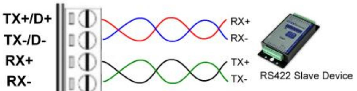
**Notice:** Due to the Hardware control problem will caused TRP-C08 under RS422/485 can't work, please take TRP-C08's RS232 screw terminal connector (RTS & CTS SHORT).
