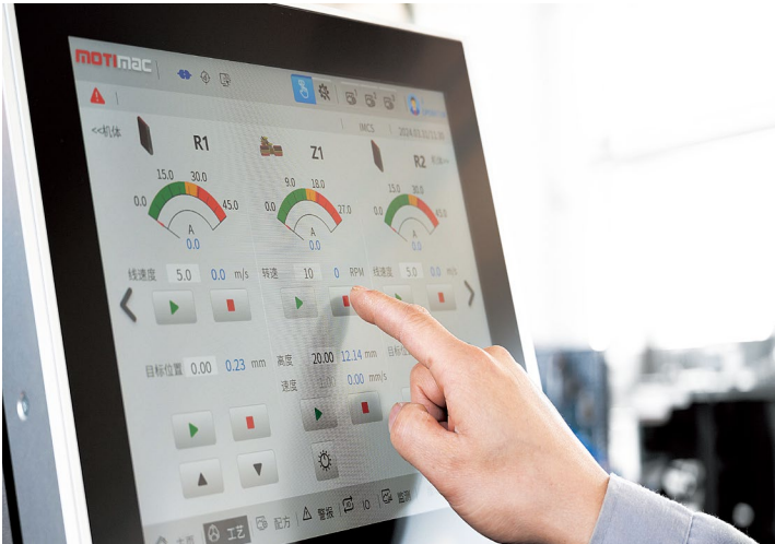
砂削量自动监测，设备出现过载时，自动停止运行，保护砂带、输送带、工件等。 Automatic stock-removal monitoring: Stops automatically during overload to protect the abrasive belt, conveyor belt, workpiece, and other components.
