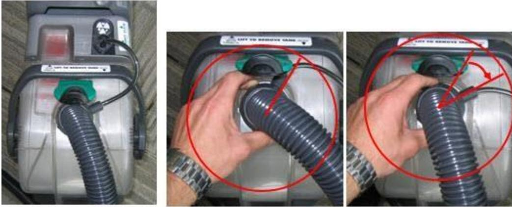
2. The hose won't suction if it's inserted incorrectly. Use the pictures below to make sure the hose is seated properly.
