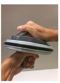
14) To reassemble, align tabs on filter piece with their mating slots on the inner cyclone and twist clockwise.
