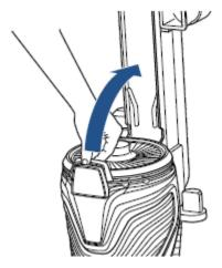
• Twist filter counter clockwise to unlock and remove
