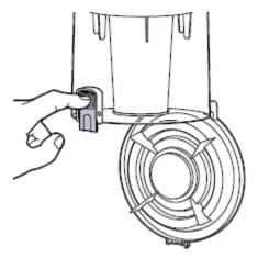
• Twist the handle to unlock the tank
