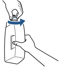
Unscrew the cap at the bottom of the Clean Water Tank.
