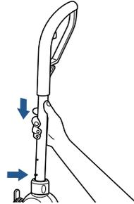
Slide upper Handle Post into the body by aligning the pin and sliding the post down into place.
