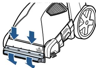
Attach the hard floor tool by hooking it into the front of the nozzle. Rotate down until it snaps into place.
