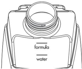
Fill with warm tap water to the WATER line. Fill the rest of the tank with BISSELL Formula to the FORMULA line.
