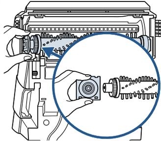
When removing the Brush Roll, the Brush Roll cap will come with it. Do not lose this part.
