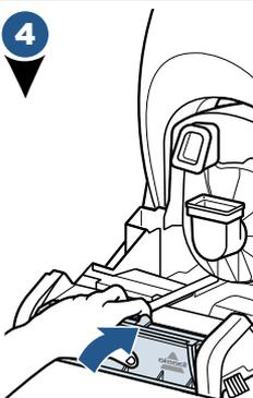
To remove and clean the nozzle, keep the Dirty Water Tank off of the machine.
