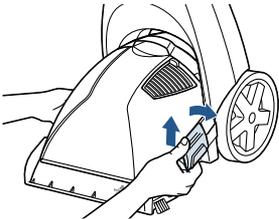
Rinse the Dirty Water Tank thoroughly and replace on machine. Secure latches on both sides of the tank.
