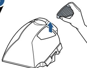
Remove tank vent & foam filter (located on top of the Dirty Water Tank) and rinse.
