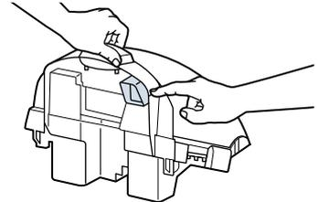
Carry the Dirty Water Tank to a sink. To empty, tilt tank and pour out contents using the opening at the back of tank.
