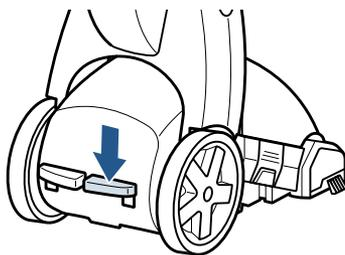
With foot, press the red Power Pedal, located on the back of the machine.
