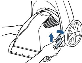
Release Dirty Water Tank Latches (on each side) by pulling up from the bottom of latch and then out.
