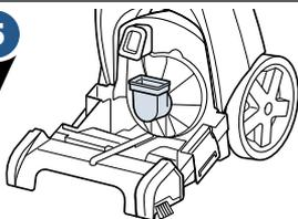
Remove lint and hair from red gasket in base of machine. (Do not remove gasket.)
