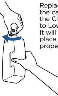
Replace and tighten the cap, then return the Clean Water Tank to Lower Body. It will “click” into place when seated properly.
