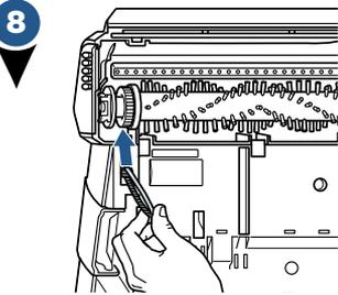
Maneuver the belt to wrap around the pulley. Wrap the belt around the cog of the Brush Roll. Secure the Brush Roll into place by sliding the square piece to align the Brush Roll.
