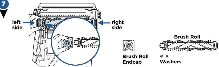
Clean or replace the Brush Roll and belt. When finished, reassemble them to the machine. Insert the brush into the right side endcap. Adjust the right side of the brush into place and tuck the left Brush Roll cap (separate piece that attaches to Brush Roll) into place.
