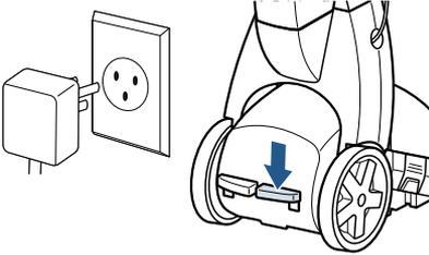
With foot, press the red Power Pedal, to turn OFF machine and then unplug.
