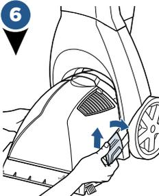
Once the parts have been rinsed clean and dried, replace the Dirty Water Tank to the base of the machine and secure with both latches. Wrap power cable around Quick Release Cable Wrap on side of the machine. Wipe all surfaces with a soft cloth and store machine upright in a protected, dry area.
