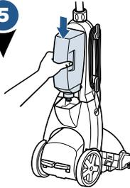
Place Clean Water Tank on back of machine, so it "clicks" into place.
