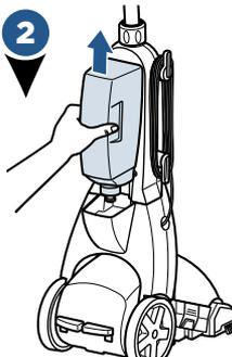
Remove the Clean Water Tank by lifting straight up and away from Lower Body. Fill the tank using water and BISSELL Wash & Shine Floor Cleaner formula for cleaning the hard floor.
