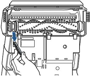
If you want to replace or clean the Brush Roll, remove the belt by slightly lifting the Brush Roll to maneuver the belt and remove it. If the belt is broken and needs to be replaced, remove it and replace with a new belt.
