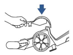
• Replace the brush cover and front nozzle to test If machine continues not to spray, contact us
