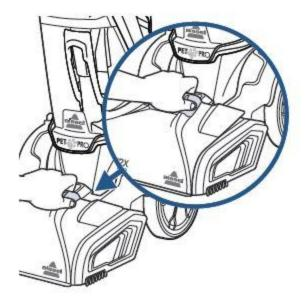
• Remove the brush roll cover by pressing the two "push" buttons
