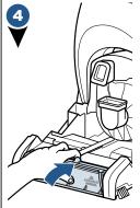
To remove and clean the nozzle, keep the Dirty Water Tank off of the machine.
