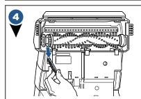
If you want to replace or clean the Brush Roll, remove the belt by slightly lifting the Brush Roll to maneuver the belt and remove it. If the belt is broken and needs to be replaced, remove it and replace with a new belt.
