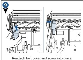
**NOTE:** Manually rotate brush to make sure it rotates freely and the belt is aligned.
