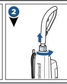
Extend the Collapsible Handle Post by turning the collar counter-clockwise and lifting the handle up. Turn the collar clockwise to secure.
