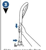
Slide upper Handle Post into the body by aligning the pin and sliding the post down into place.
