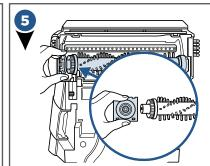
When removing the Brush Roll, the Brush Roll cap will come with it. Do not lose this part.
