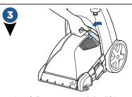
Carefully remove tank by lifting up on the Carry Handle.
