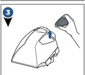
Remove tank vent & foam filter (located on top of the Dirty Water Tank) and rinse.
