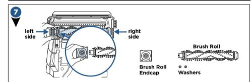
Clean or replace the Brush Roll and belt. When finished, reassemble them to the machine. Insert the brush into the right side endcap. Adjust the right side of the brush into place and tuck the left Brush Roll cap (separate piece that attaches to Brush Roll) into place.
