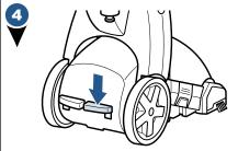
With foot, press the red Power Pedal, located on the back of the machine.
