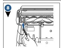
Maneuver the belt to wrap around the pulley. Wrap the belt around the cog of the Brush Roll. Secure the Brush Roll into place by sliding the square piece to align the Brush Roll.
