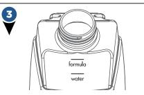
Fill with warm tap water to the WATER line. Fill the rest of the tank with BISSELL Formula to the FORMULA line.
