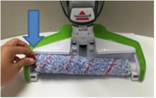
• Reattach the brush roll window by lining up the tabs on the front edges of the foot and then pushing the window into place until it clicks into place.
