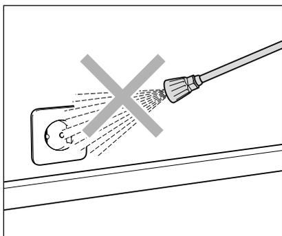
Never direct the high pressure jet at power sockets or any other electrical installations!
