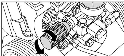
13. Adjust operating pressure infinitely using the rotary handle. The maximum pressure is factory-set.
