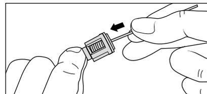
Do not forget the O-ring during reassembly!
