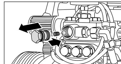
Remove check body and check O-Ring for soiling or damage. Also check seal seat inside pump housing for soiling or damage.
