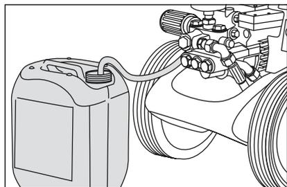
1. Place chemicals filter into container with additives.
