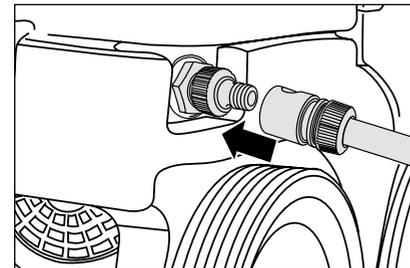
8. Connect the water hose to water inlet sieve. The high pressure cleaner may be connected to a water mains (1-10 bar pre-pressure) with either cold or hot water (up to 60 °C). The small quadro series provides the opportunity of sucking in water out of a container (see direct suction).
