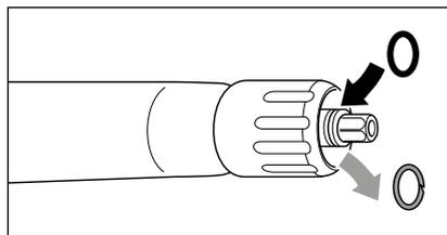
Switch off the high pressure cleaner. Shortly press the trigger of the safety trigger gun to decrease the high pressure cleaner. Unscrew high pressure hose, safety trigger gun and lance and check the O-rings. If the O-rings are damaged they have to be replaced.
