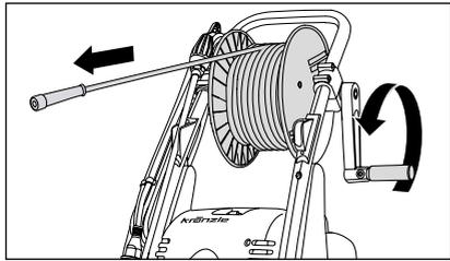
3. Release fixation of hose drum. Unwind high pressure hose straight and without nooses. Completely unwind hose. The high pressure hose may leave signs of abrasion on some floors. Alternatively, please also find non-marking high pressure hoses in our range.
