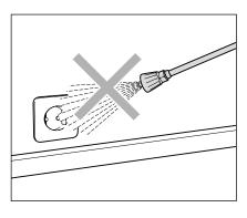
Never direct the high pressure jet at power sockets or any other electrical installations!
