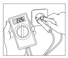
If there are too many collectors in your proximity connected to the network at the same time, the available voltage and the current intensity may decline. Consequently the motor of the high pressure cleaner does not start or even blows. The power supply may also be insufficient if the power supply cable is too long or too thin. If extension cables are too long, this may lead to a voltage drop causing malfunctions or start-up difficulties.
