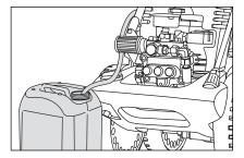
Place chemicals filter into container with additives
