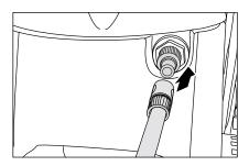
8. Connect the water hose to water inlet sieve. The high pressure cleaner may be connected to a water mains (1-10 bar pre-pressure) with either cold or hot water (up to 60 °C). The medium quadro series provides the opportunity of sucking in water out of a container (see direct suction).
