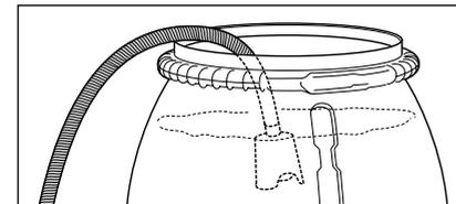
3. Put filled suction hose into the water-filled container and start the cleaning job. **Use clean water only! Never suck in water containing chlorine! Do not suction air!**
