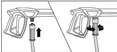
4. Tightly screw together high pressure hose and safety trigger gun.
