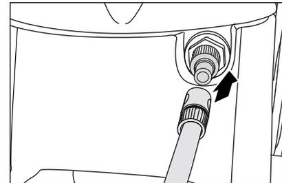
8. Connect the water hose to water inlet sieve. The high pressure cleaner may be connected to a water mains (1-10 bar pre-pressure) with either cold or hot water (up to 60 °C). The medium quadro series provides the opportunity of sucking in water out of a container (see direct suction).
