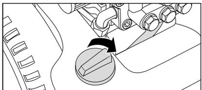
2. Dosing of detergent is done by turning the detergent valve.
