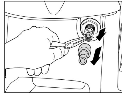
7. **Check water inlet filter for cleanliness prior to putting the high pressure cleaner into operation.**
