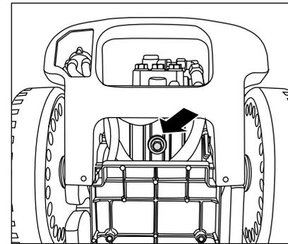
The first oil change should be carried out after approximately **50 operating hours**, then every year or after 250 operating hours. If the oil turns grey or white, you must change the oil. In case of exchanging oil being required, the oil drain screw must be opened above a container and the high pressure cleaner be emptied. The oil is to be caught in the reservoir and disposed of in an approved manner.
