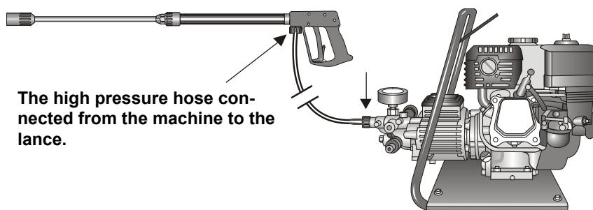
The high pressure hose connected from the machine to the lance.
