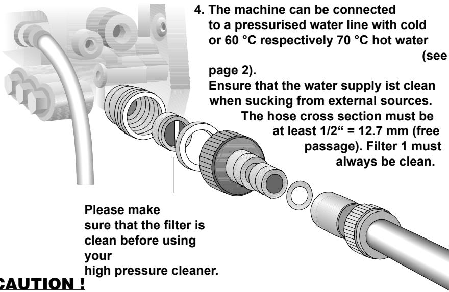
4. The machine can be connected to a pressurised water line with cold or 60 °C respectively 70 °C hot water (see page 2).
