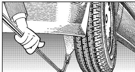
Underbody cleaning of cars, trailers and equipment: lance 90 cm with high pressure nozzle and ST 30 nipple. The lance must be aimed when spraying.
