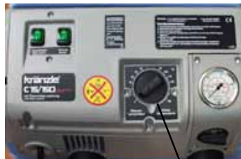
Thermostat with rotary control switch
