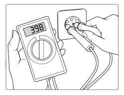
If there are too many collectors in your proximity connected to the network at the same time, the available voltage and the current intensity may decline. Consequently the motor of the high-pressure cleaner does not start or even blows. The power supply may also be insufficient if the power cable is too long or too thin. If extension cables are too long, this may lead to a voltage drop causing malfunctions or start-up difficulties.
