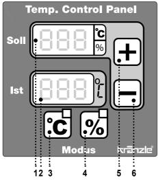
The thermostat controls the spray water temperature.
