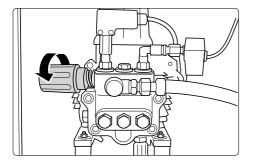
The pressure control valve on the pump head is used to control the operating pressure plus the water flow and consequently the water temperature as well. Turn right to increase the pressure, turn left to reduce the pressure.
