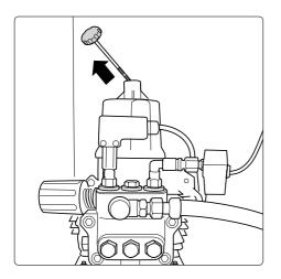
**6.** Always check oil level prior to operation! Open the machine.
