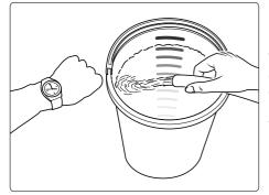
Lack of water occurs more often than you probably believe. The more powerful a highpressure cleaner is the greater is the danger that a lack of water occurs. If there is only an insufficient amount of water available, cavitation arises inside the pump, which is normally noticed too late or even not at all. The pump will be destroyed. Please check the available quantity of water by filling a bucket with litre scale for one minute.
