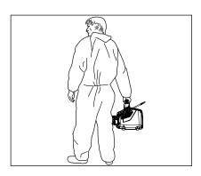
Carry the K 1050 P to its place of operation. When parking the highpressure cleaner make sure that the four rubber buffers stand on a safe support.
