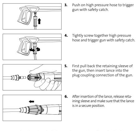
Prior to insertion, check plug coupling connection of lance for cleanliness (sand, dirt ..) and use clear water to clean, if necessary. Impurities may damage the sealing in the plug coupling.
