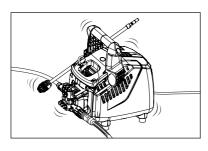
Having closed the trigger gun with safety catch, the HP cleaner must shut down. Failure to shut down may be caused by leakage in the pump, the pressure switch, the high pressure hose or the trigger gun with safety catch.
