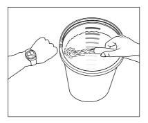
Lack of water occurs more often than you probably believe. The more powerful a high-cleaner is the greater is the danger that a lack of water occurs. If there is only an insufficient amount of water available, cavitation (water-gas mixture) arises inside the pump, which is normally noticed too late or even not at all. **The pump will be destroyed**. Please check the available quantity of water by filling a bucket with liter scale for one minute.
