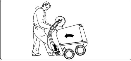
1. Steering the machine: To change direction tilt machine by pressing a foot against the footrest and pull the handle at the same time. Then turn machine into desired direction.
