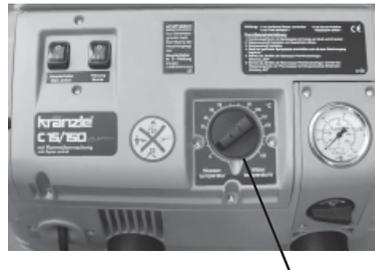
Thermostat with rotary control switch
