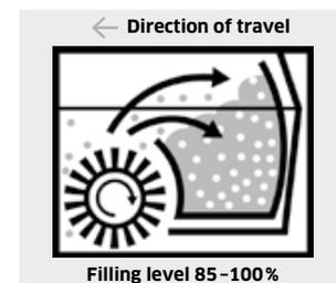
Effective: high-speed sweeping principle fills dirt hopper 100%.
