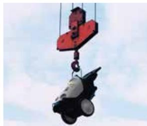
Loading is no problem: suitable for cranes thanks to lifting points.
