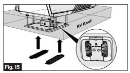
15. Align the decoration plate tabs with the mating notches on the ADB shroud and push to snap the decoration plate into place. (Fig. 16)
