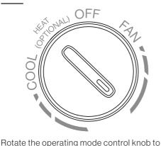
the "HIGH FAN" mode position (as shown above), and keep the air conditioner running for half an hour. Then the frost and ice will be melted and drop down of the evaporator coil, and the air conditioner will be resumed.
