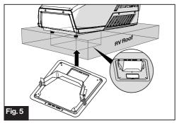
5. Fix the assembled mounting frame and lower duct divider into the rooftop unit using 4 bolts provided. (Fig. 6)
