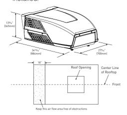
Check the inside of the RV for return air kit obstructions. (i.e. door openings, room dividers, curtains, ceiling fixtures, etc.) Allow 6" (152mm) space from the opening to account for any potential return air kit obstructions.
