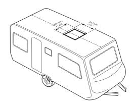
2. Using the roof opening as a guide, cut a matching hole in the ceiling.
