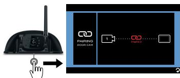
5. Repeat the steps to pair the other available cameras. Erect antennas (if available) on both the monitor and camera(s). Ensure the signal strength is OK.
