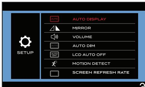
2. Tap the **AUTO DISPLAY** switch to highlight it red and enable this function. Here, you can tap **QUAD-View** to enter
