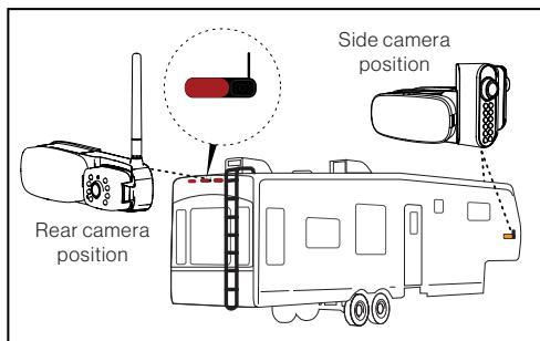
2. Remove the lens cover and detach the camera from the marker light bracket (right side camera shown).
