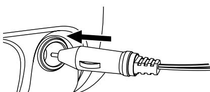
4. Connect the DC connector to the power socket on the monitor.
