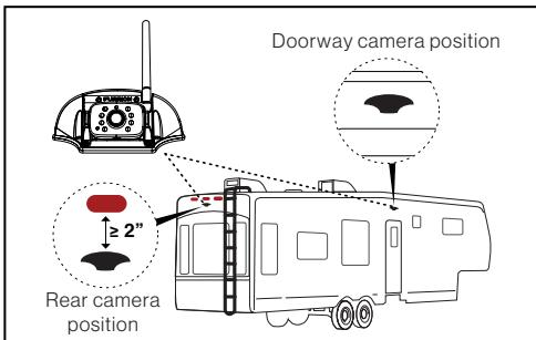
2. Use the gasket as a template to mark a basic outline on the chosen location with a pencil. Drill a 5/8" center hole. Then route the female connector of the camera power cable through the hole and leave 2 inches of slack.
