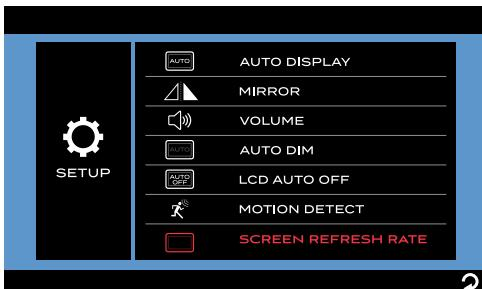
2. Tap to set the screen refresh rate to **60Hz** or **50Hz**.
