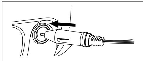
4. Connect the DC connector to the power socket on the monitor.
