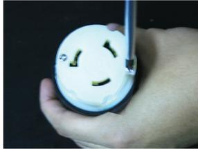
2. Remove the threaded cable strain relief piece from the rear cover.
