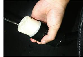
7. From step #3, slide in the strain relief components 2 and 3 to the rear of the connector cover, then push the threaded strain relief (1) to secure and tighten the nut using a 1½" wrench until the cable is gripped. Do not over tighten.
