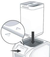
Press the **PRESS AND RELEASE** button on the power station and pull upwards on the battery handle to remove the battery.
