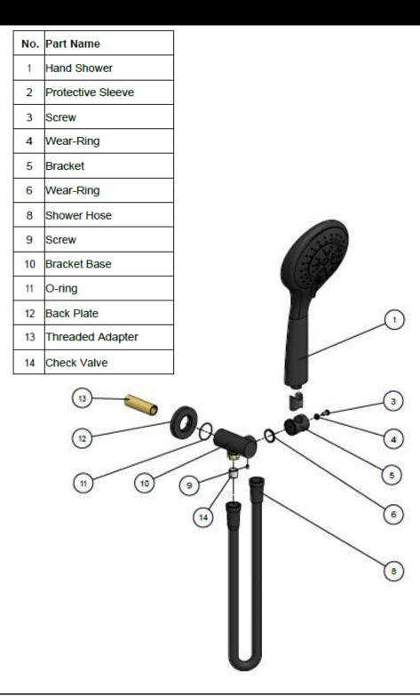
NOTE: The hose end caps of parts (7,8) are made from a special hardened plastic to prevent the brass mount (5) from scratching.
