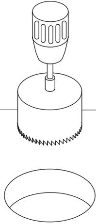
Drill out a 2 ½" diameter hole to fit the threaded base column.
