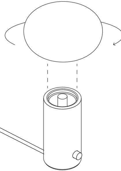
Attach the diffuser to the lamp base by rotating clockwise until fixed in place
