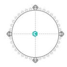
Attach the springs to the jump mat Attach the more tightly curled end of the springs to the D-rings on the jump mat.
