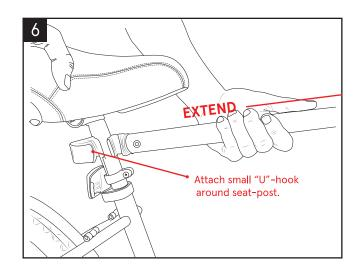
Lift up and down to make sure the Top-Tube Adapter is securely attached to the bike.
