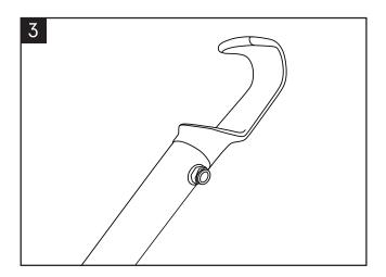
**5.** Attach the large U-shaped yoke to the handlebar stem, insert the clevis pin completely through the two holes in the yoke, making sure the retainer clip is properly closed.
