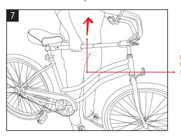
**4.** Make sure the handlebar stem and seat post are tightly attached to the bicycle, and the seat securely attached to the seat post.
