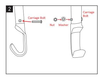
**3.** Screw nut onto the Carriage Bolt and tighten to make the nut flush with the screw.
