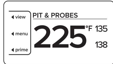
As shown in Section 1.C, the “Pit & Probes” view is the default display option. There are five total display options; they can be chosen by pressing the view selection button on the control panel.
