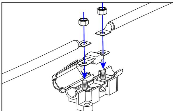
REDARC offer MIDI fuse kits containing the required fuses, fuse holders, crimps and nuts:
