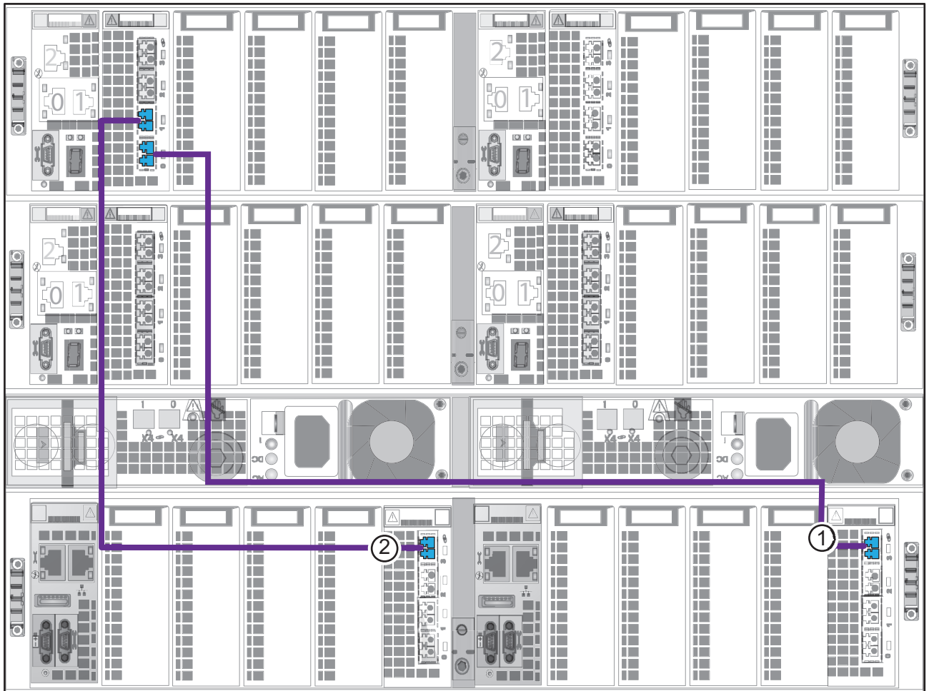
Figure 35 Cable storage processors to blade 5
