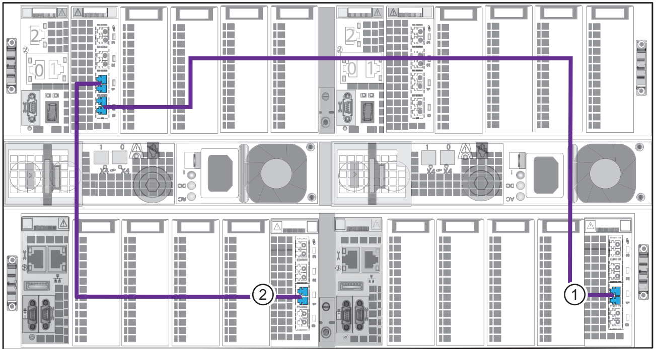
Figure 33 Cable storage processors to blade 3
