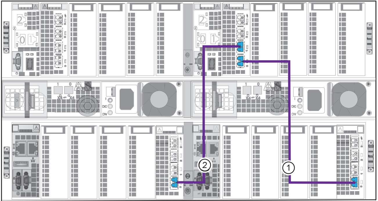
Figure 32 Cable storage processors to blade enclosure 0
