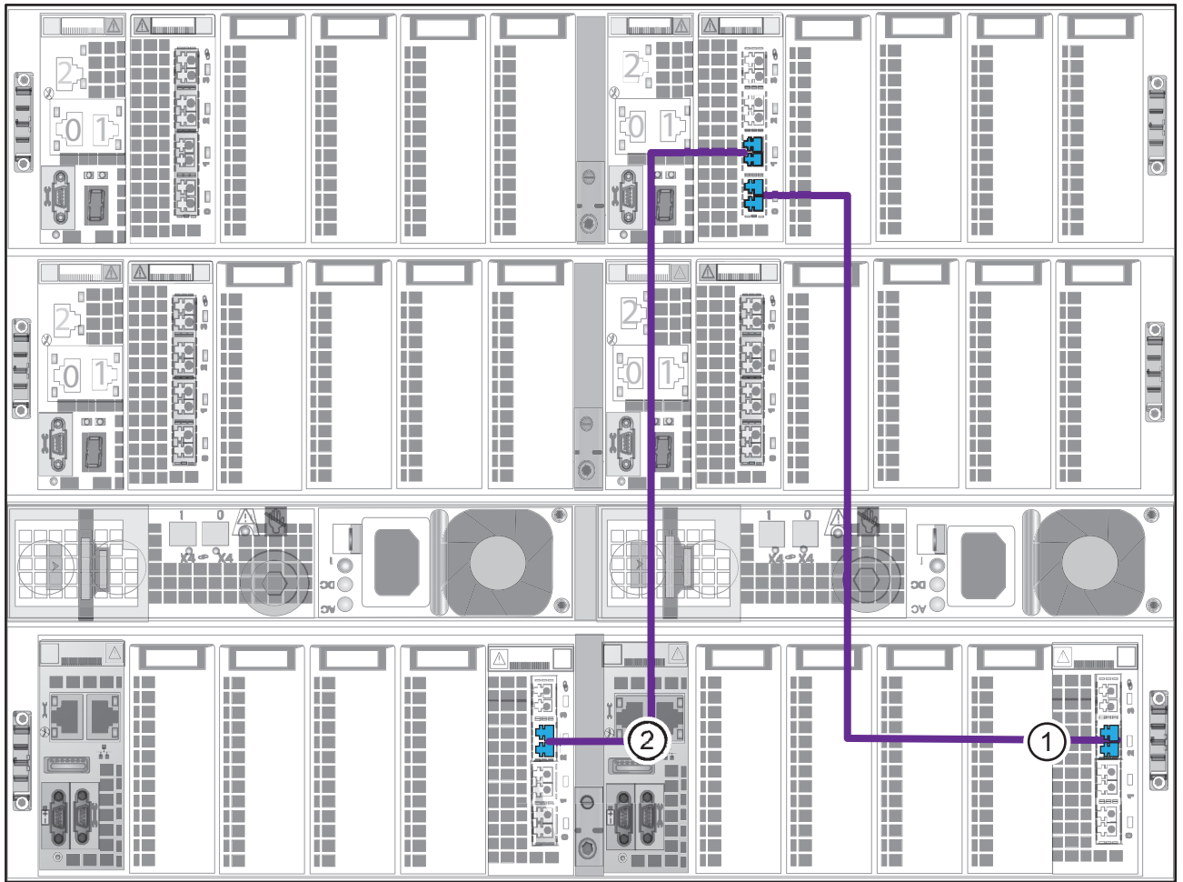
Figure 34 Cable storage processors to blade 4
