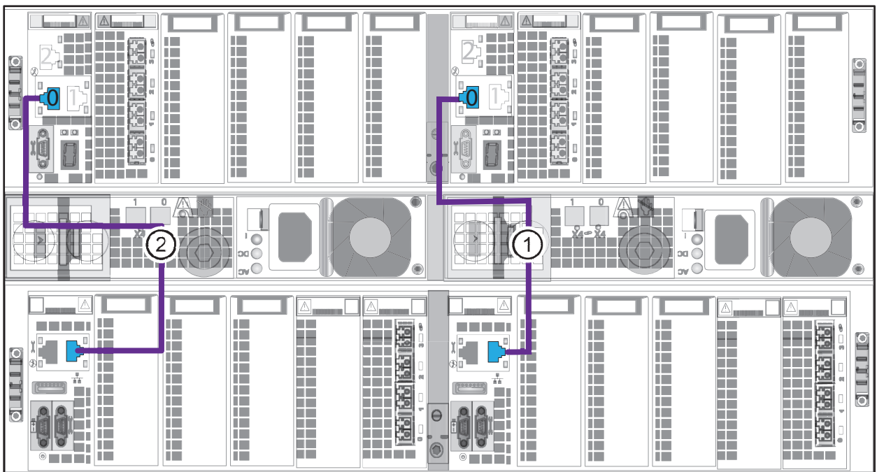
Figure 41 Cabling SPs to blade enclosure 0
